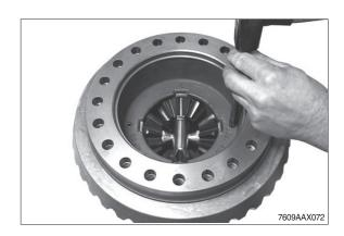
$\ensuremath{{\ensuremath{\bigcirc}}}$  Mount second axle bevel gear.
