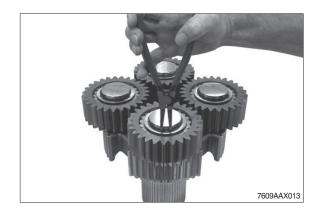
Pull off planetary gear.
