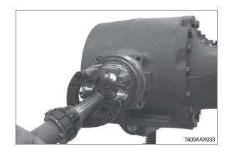
⑤ Loosen slotted nut and remove the shim behind.
