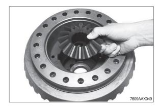
Press crown wheel from the differential carrier.
