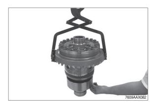
Preload the differential by means of the press and the pressure piece.
