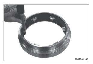
⑤ Insert the piston into the brake housing and carefully install with the fixing device until contact is obtained.
